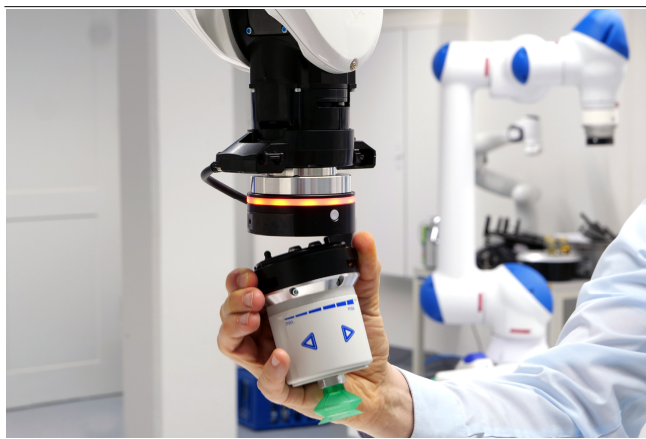
Quick-change module RMQC for manual gripper changes
